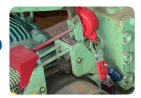
for The Control of Hazardous Energy (Lockout/Tagout) (29 CFR 1910.147) for general industry outlines measures for controlling different types of hazardous energy. The LOTO standard establishes the employer's responsibility to protect workers from hazardous energy. Employers are also required to train each worker to ensure that they know, understand, and are able to follow the applicable provisions of the hazardous energy control procedures:
